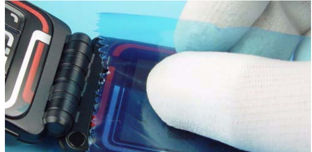
2.) Open the unit and protect the window of the Inner LCD with a plastic film.
