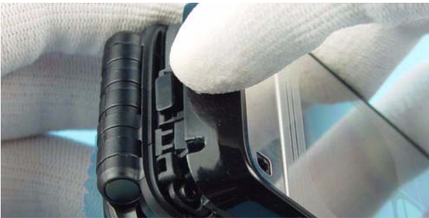
3.) Press the release button and remove the B-Cover Lower Assy .
