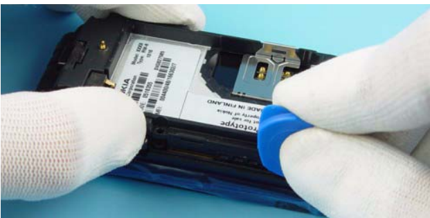
5.) Use the SRT-6 as a lever to open the snaps of the C-Cover .
