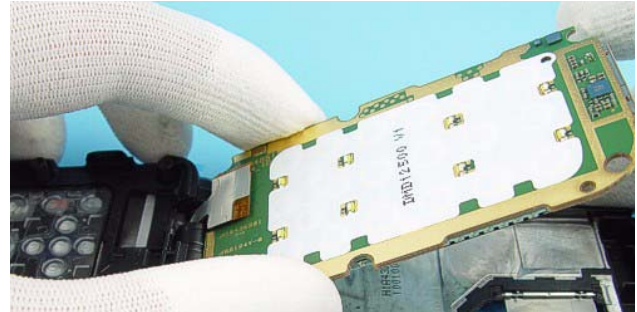
12.) Turn the Engine Module as shown in the picture. Use the C-Cover Assy as support for Engine Module .
